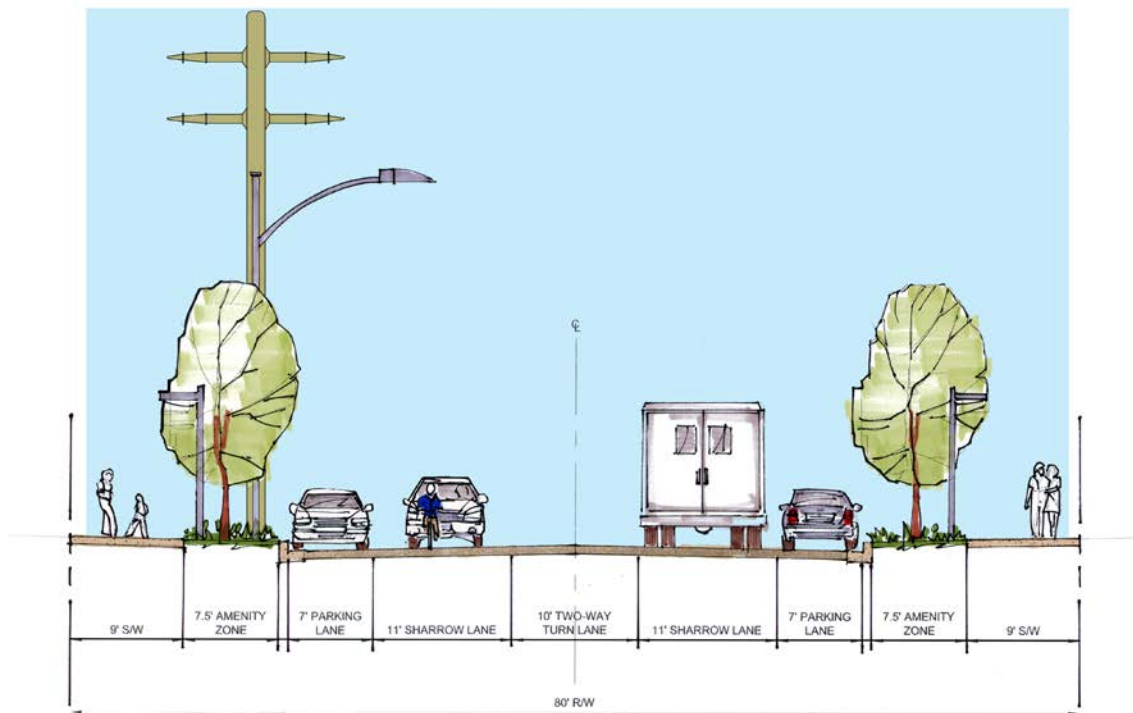
PROPOSED TYPICAL SECTION LOOKING WEST JERROLD AVE
