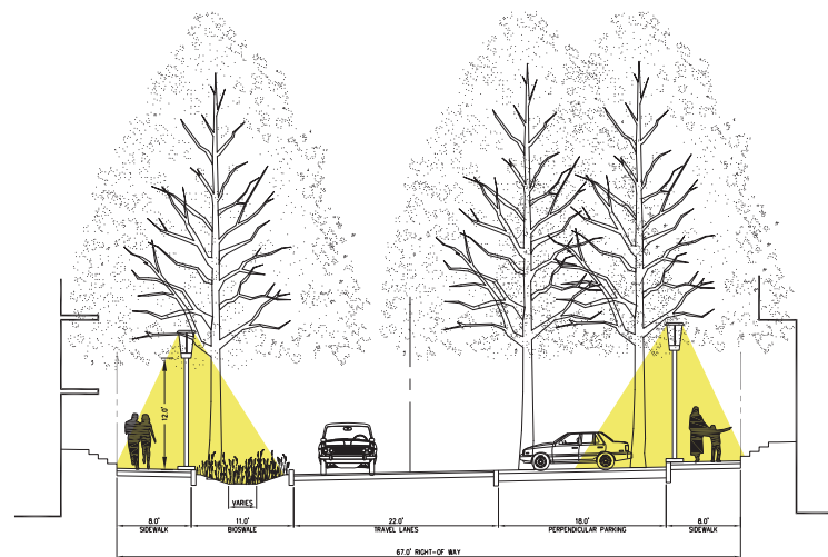
Residential lighting typical section
