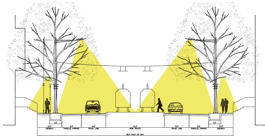
Boulevard lighting typical section
