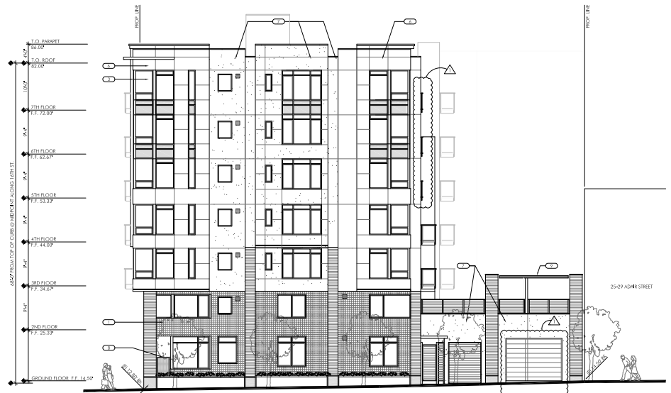
Figure 16: North Exterior Elevation - Adair St.
