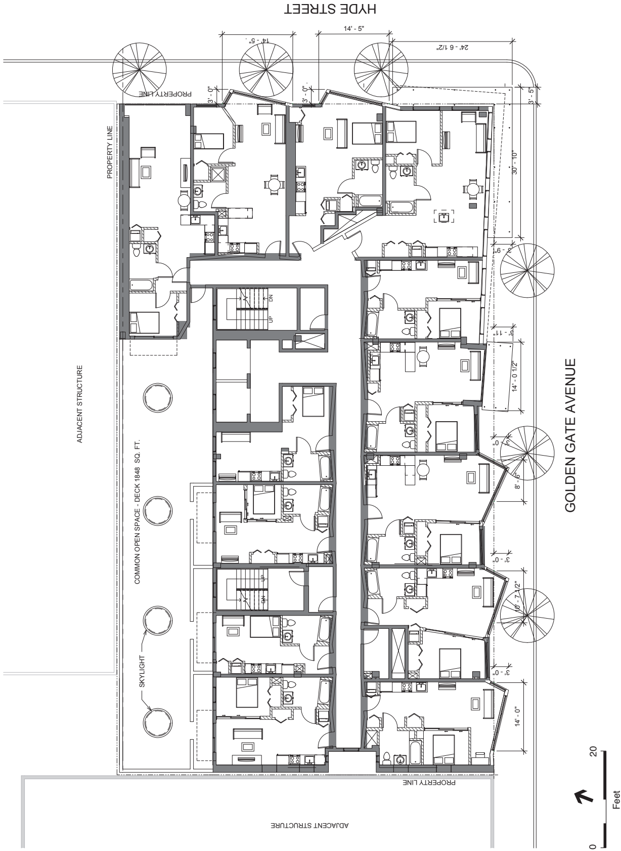
2012.0086E: 101 Hyde Street Figure 5 Proposed Second-Floor Plan
