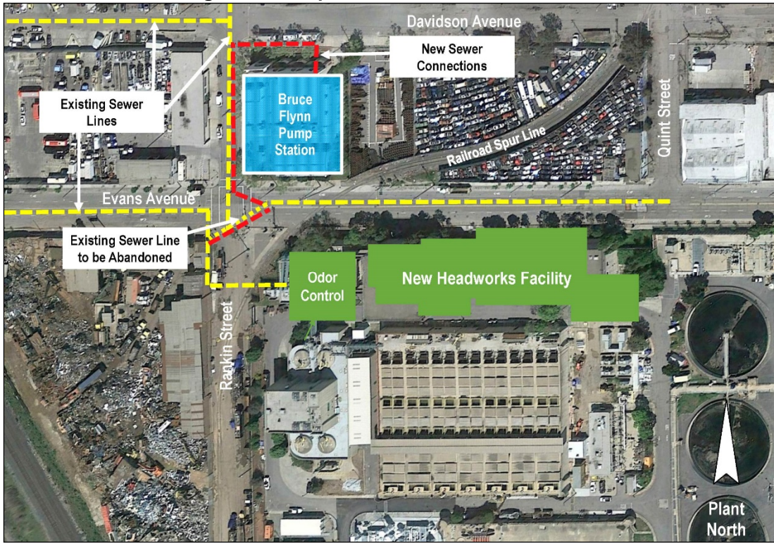
Figure 10: Proposed BFS Sewer Connection
