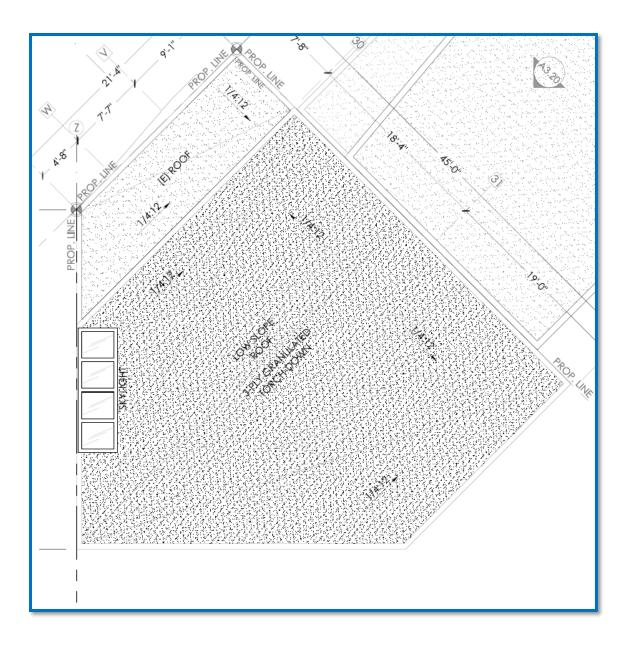
Figure 18: Roof Plan for Lot 35B
