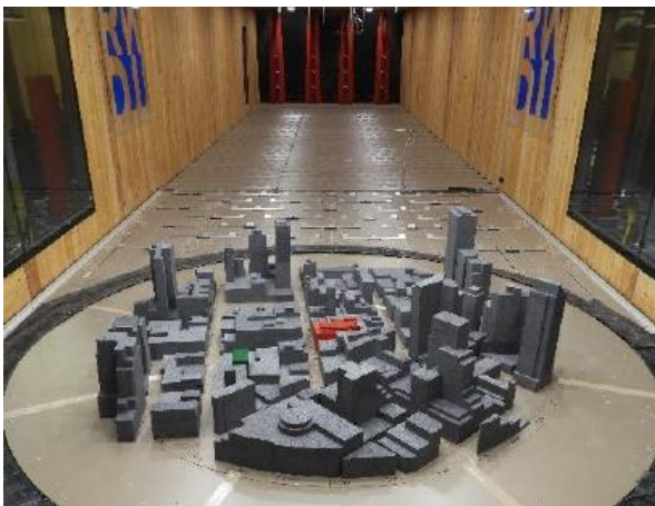
Image 8: Photos of wind tunnel models of select projects along Market Street (1028 Market Street – top left, First and Mission – top right, 120 Stockton Street – bottom left & 30 Van Ness – bottom right)
