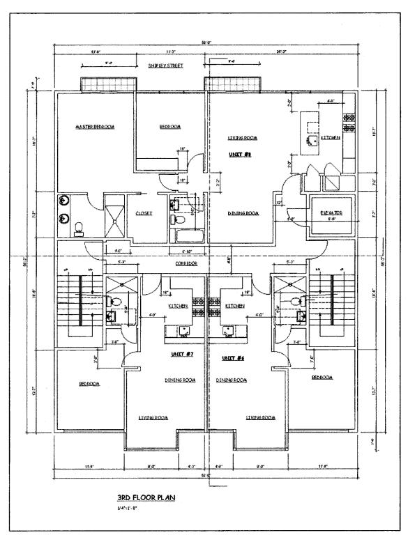
Figure 5. Proposed third floor plan (Source: William Pashelinsky Architect)
