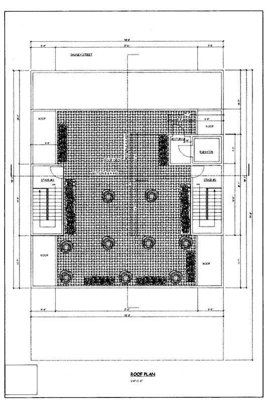
Figure 7. Proposed roof plan (Source: William Pashelinsky Architect)
