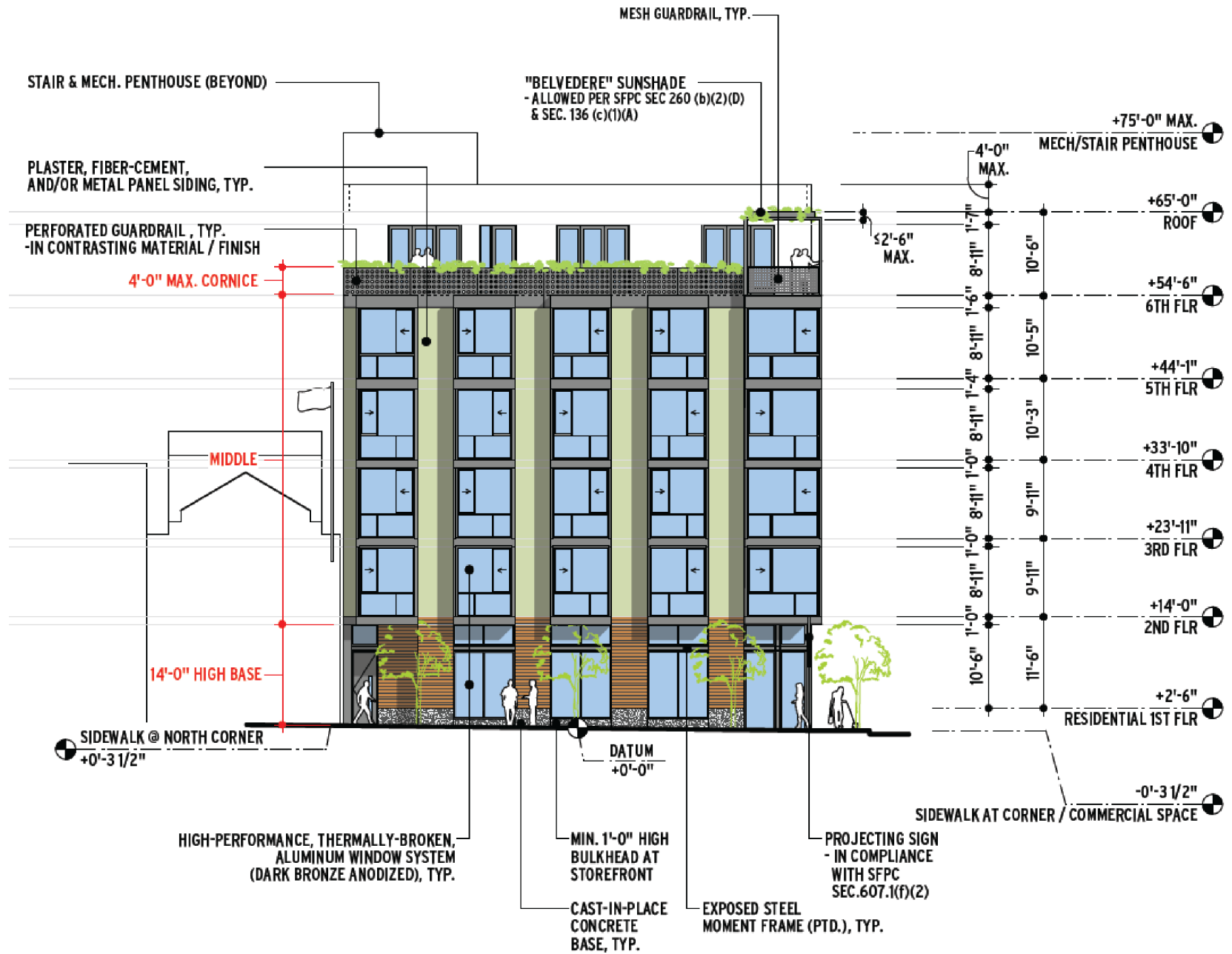
Figure 6 - West (Dore Street) Building Elevation
