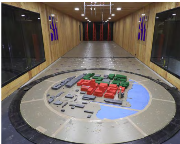
Image 2c: Wind Tunnel Study Model – Project + Cumulative Configuration
